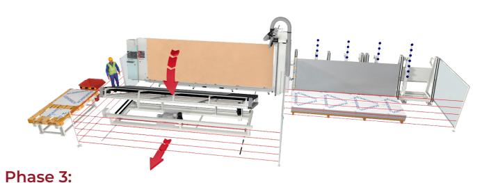
Off Loader returns into horizontal position while moving back away from the panel router. Once the light curtains are unenganged the Alu Ranger commands Alu Feeder to load the next panel. During this phase Alu Ranger and Alu Loader safety light curtains are active.
